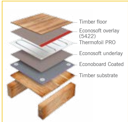
Typical floating floor build up
