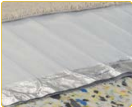
5415 Vapour Barrier Vapour Barrier is an alternative to Econosoft Overlay where the acoustic properties are not required (such as under carpet) and acts to inhibit the transfer of any moisture that may be present in the substrate from being absorbed into the floor finish. Either Econosoft or Vapour Barrier must be installed above Thermofoil PRO in every installation.
