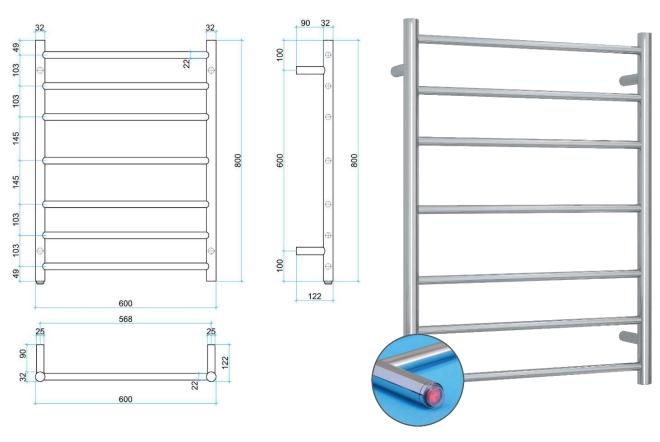
This rail has Multiflex wiring which means that there is a connection point on both the left and right hand side of the rail and the lead can be connected to either side. Being a dry electric element rail, this can be mounted either way up meaning the wiring can be from any of the four mounting points.
