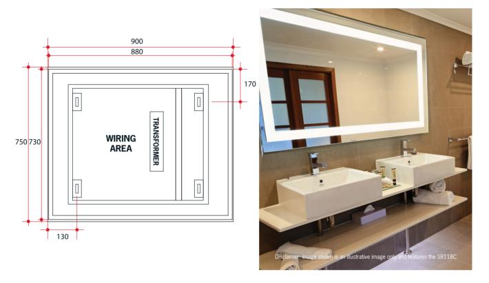
Note: All dimensions are in millimetres (mm)
