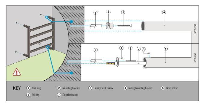
The Thermorail models in this guide can only be installed with concealed wiring (Hardwired), with the electrical connection on either the right or left hand side.
