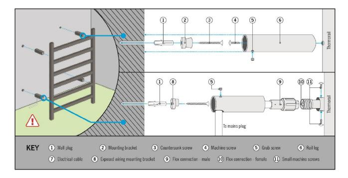
The Thermorail models in this guide can be installed with either concealed or exposed wiring, with the electrical supply connected at the bottom or top, left or right hand mounting point. This section concentrates on the exposed wiring method. For concealed wiring see page 4.
