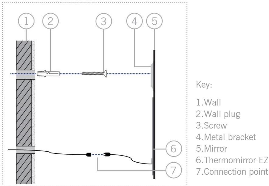
When installing the Thermomirror EZ demister with a hanging mirror the demister pad needs to be adhered directly to the back of the mirror. The Thermomirror EZ demister cannot be cut or pierced. Before starting installation ensure the Thermomirror demister size is suited to the size of the mirror and that it will not cover any fixings or hangers.
