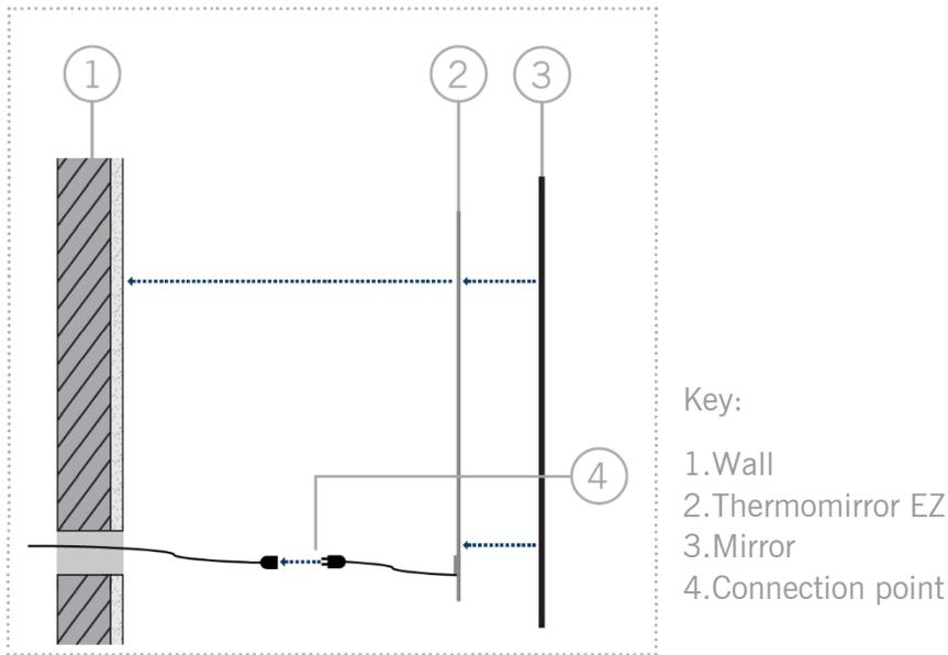
When installing the Thermomirror EZ demister with a glue-to-wall mirror there needs to be 100mm spacing all around the Thermomirror to allow for sufficient adhesion between the mirror and the wall.
