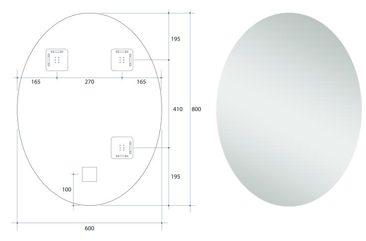
Note: All dimensions are in millimetres (mm)
