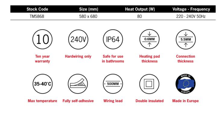
Thermomirror demisters must be installed by a qualified electrican. The demister cannot be cut, pierced or modified in anyway.
