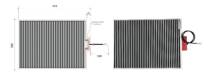
Note: All dimensions are in millimetres (mm)
