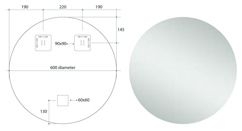
Note: All dimensions are in millimetres (mm)
