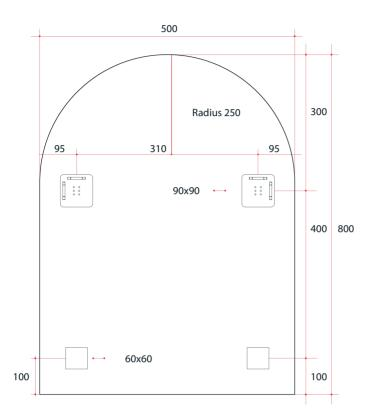
Note: All dimensions are in millimetres (mm) The depth of the mirror is 5mm, the space between the back of the mirror and the wall due to the hangers is 9mm making the total depth 14mm.
