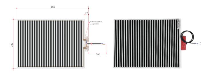
Note: All dimensions are in millimetres (mm)
