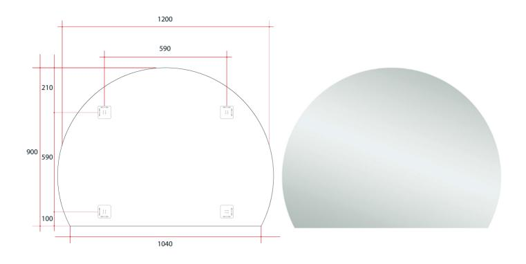
Note: All dimensions are in millimetres (mm)
