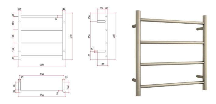
Note: All dimensions are in millimeters (mm)
