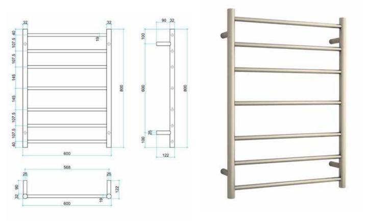
This rail has Multiflex wiring which means that there is a connection point on both the left and right hand side of the rail and the lead can be connected to either side. Being a dry element rail, this can be mounted either way up meaning the wiring can be from any of the four mounting points.
