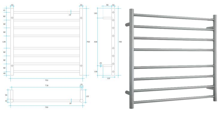
Note: All dimensions are in millimetres (mm)
