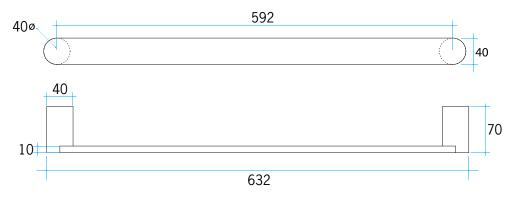
Note: All dimensions are in millimetres (mm)
