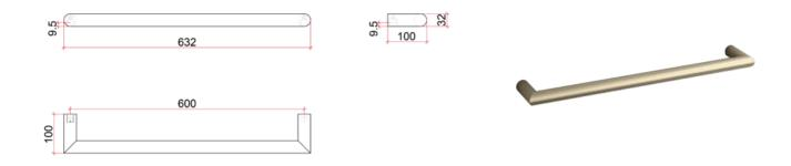
Note: All dimensions are in millimeters (mm)
