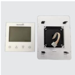
This will release the main unit from the mounting plate and then you will need to unclip the ribbon cable from the back of the screen.
