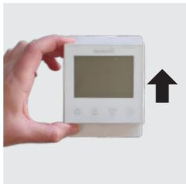
Remove the Thermostat from the box and press upwards on the main square unit.
