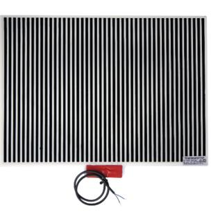
Stock Code Size (mm) Heat Output (W) Voltage - Frequency TM3545 350 x 450 38 220 - 240V 50Hz  $\downarrow$ IP64 0.6MM 240 5.5MM  $\uparrow$ Safe for use **Heating pad** Connection Ten year Hardwiring only warranty in bathrooms thickness thickness 500MM 35-40°C **Max temperature Fully self-adhesive** Wiring lead **Double insulated** Made in Europe
