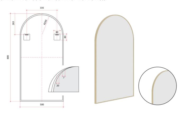
Note: All dimensions are in millimetres (mm)
