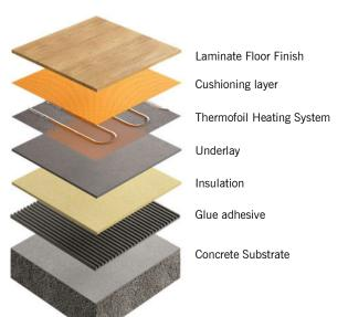
This build-up is showing a laminate floor finish on top of a Thermofoil heating mat. The Heating is laid on top of the underlay and has a cushioning layer on top. The insulation is fixed using glue adhesive.
